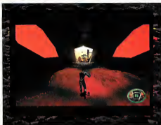
CON-VIRGE-ANCE The transparency test failed (red zones) and anti-aliasing (jaggies on the doorway) didn't work well on MDK with the VIRGE card.
